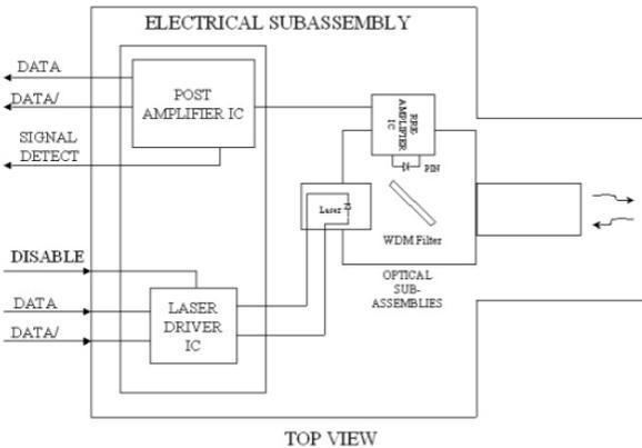
**Transmitter and Receiver Optical Sub-assembly Section** - A 1310 nm InGaAsP laser and an InGaAs PIN photodiode integrate with an WDM filter to form a bi-directional single fiber optical subassembly (OSA). The laser of OSA is driven by a LD driver IC which converts differential input LVPECL logic signals into an analog laser driving current. The photodiode of OSA is connected to a circuit providing post-amplification quantization, and optical signal detection.
